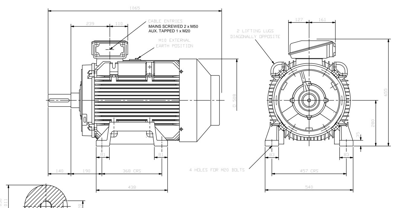
TERMINAL BOX CAN BE SIDE MOUNTED (LEFT OR RIGHT) BY REFITTING FEET 90° IN APPROPRIATE DIRECTION.
